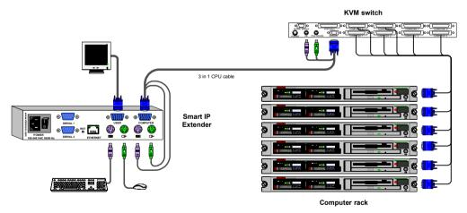
Figure 6 IP Extender connections to a KVM switch
